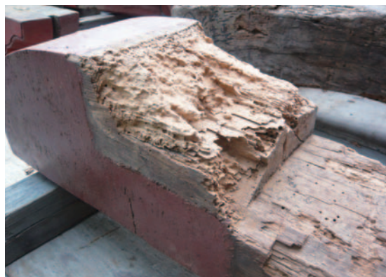
シバンムシに食害された部材 Wood member damaged by anobiid
